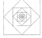
stresses, the tower was rebuilt with a rotation of 45° in order to transfer these from the corners to the central walls, which had the support of the roofs and walls of the transepts and choir. The upper portion fits well and succeeds in reducing its mass, and time has proved that the remedy worked.
