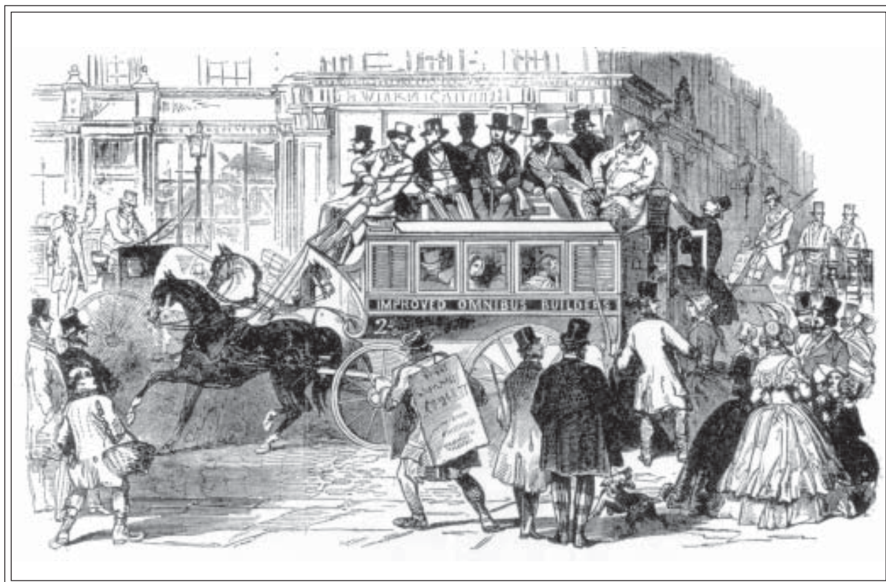
The improved omnibus introduced in April 1847. Its clerestory roof provided longitudinal seating. Illustrated London News 1 May 1847
